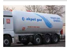
34 m³ EN12493-TPED-ADR Certification with Pump (shaft driven) and Meter
