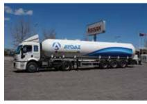
45 m³ 3 Axles Air Suspension
