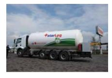
34 m³ EN12493-TPED-ADR Certification with Pump (shaft driven) and Meter
