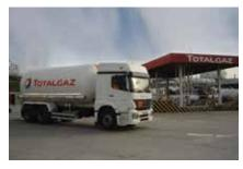
23 m³ EN12493-TPED-ADR Certification with Pump (Hydraulic driven) and Meter
