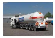
45 m³ 3 Axles Air Suspension
