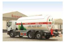
23 m<sup>3</sup> EN 12493-TPED-ADR Certification with Pump (shaft driven) and Meter
